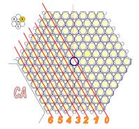
Power peak is effectively mitigated by Hf pins in the NOVCD design **Verified by Core Simulator calculations**
