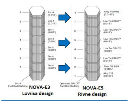
Design changes focus on increase of grid-to-rod-fretting resistance
