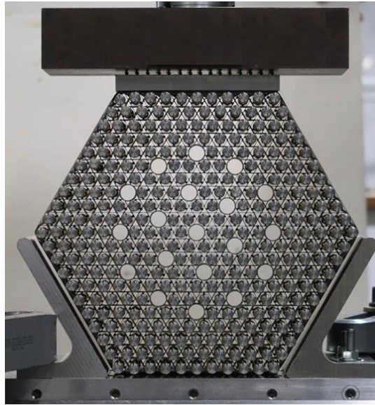
Figure 3.5 Lateral Scoping Test Setup
