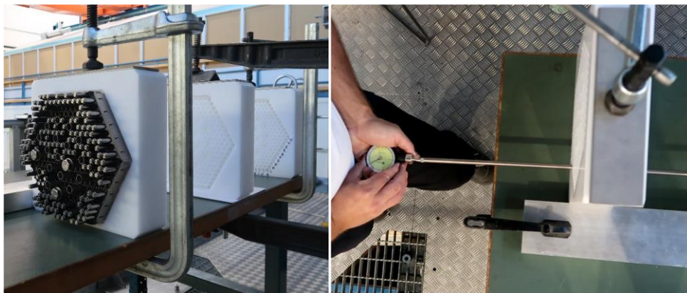
Figure 3.6 Rod Loading Test Setup
